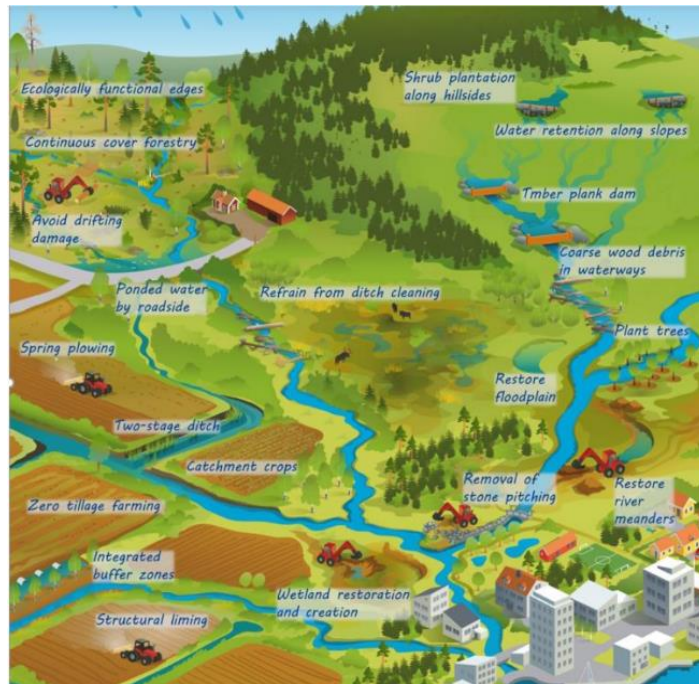
Figure 1: NbS for lowering flood risk in different river sections. Adapted from the Norwegian Environment Agency 2
