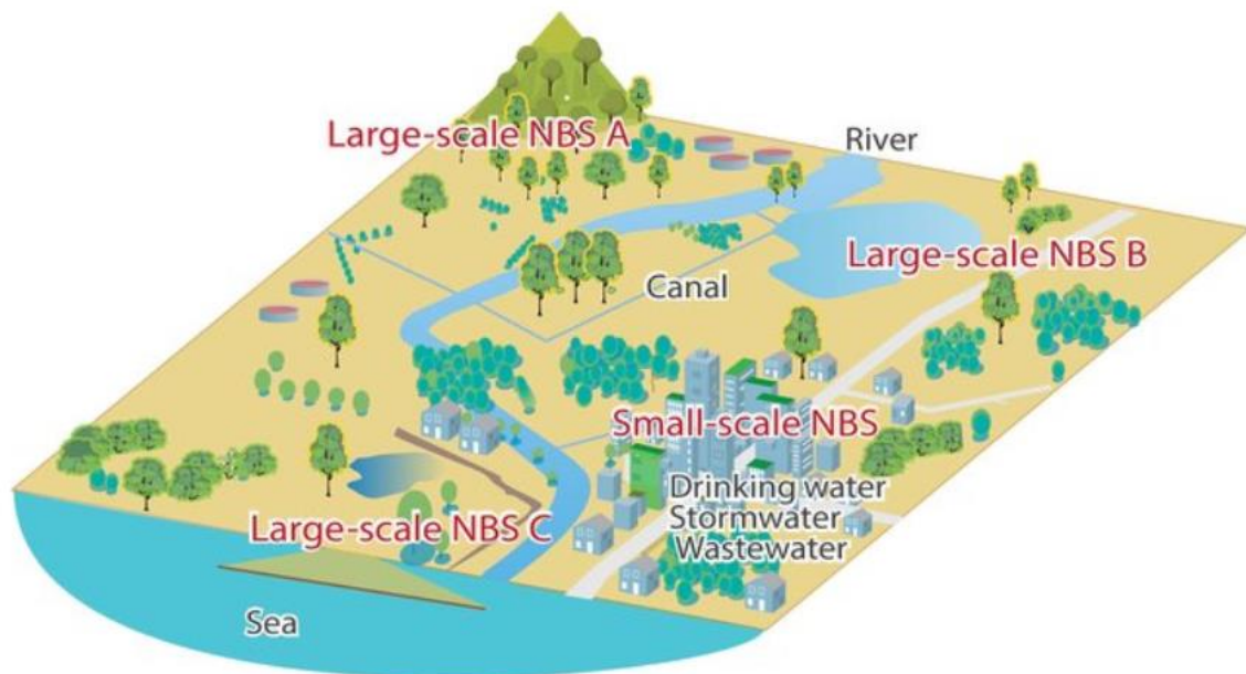
Figure 1: Illustration of large and small-scale Nature-based Solutions (NbS). Large-scale NBS A in mountainous regions (e.g. afforestation) B along river corridors (e.g. retention basins) and C in coastal regions (sand dunes) to complement small-scale NbS like green roofs etc. 2
